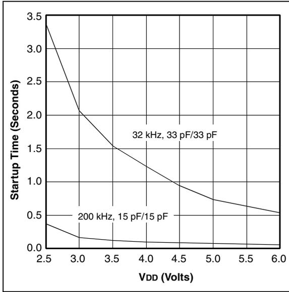
**FIGURE 14-24: TYPICAL XTAL STARTUP TIME vs. VDD (XT MODE, 25°C)**
