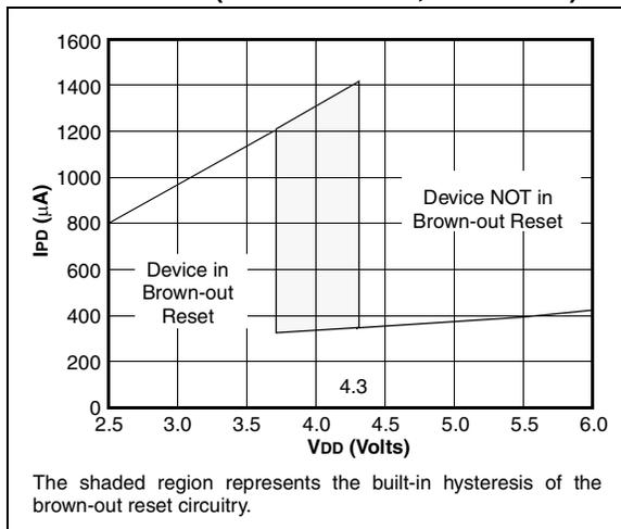
**FIGURE 14-10: TYPICAL I<sub>PD</sub> vs. TIMER1 ENABLED (32 kHz, RC0/RC1 = 33 pF/33 pF, RC MODE)**
