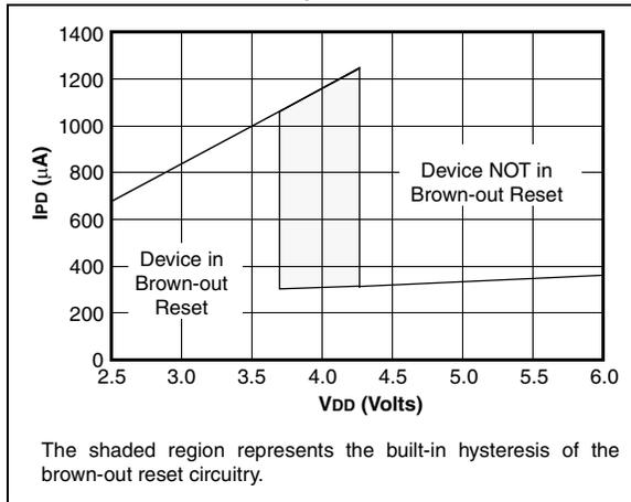
**FIGURE 14-9: MAXIMUM I<sub>PD</sub> vs. V<sub>DD</sub> BROWN-OUT DETECT ENABLED (85°C TO -40°C, RC MODE)**
