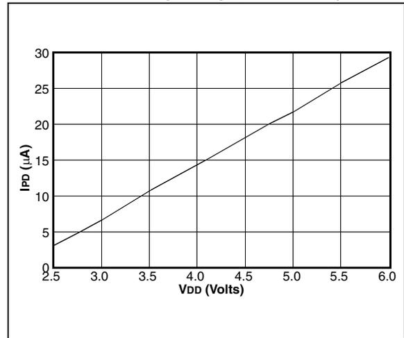
**FIGURE 14-11: MAXIMUM I<sub>PD</sub> vs. TIMER1 ENABLED (32 kHz, RC0/RC1 = 33 pF/33 pF, 85°C TO -40°C, RC MODE)**
