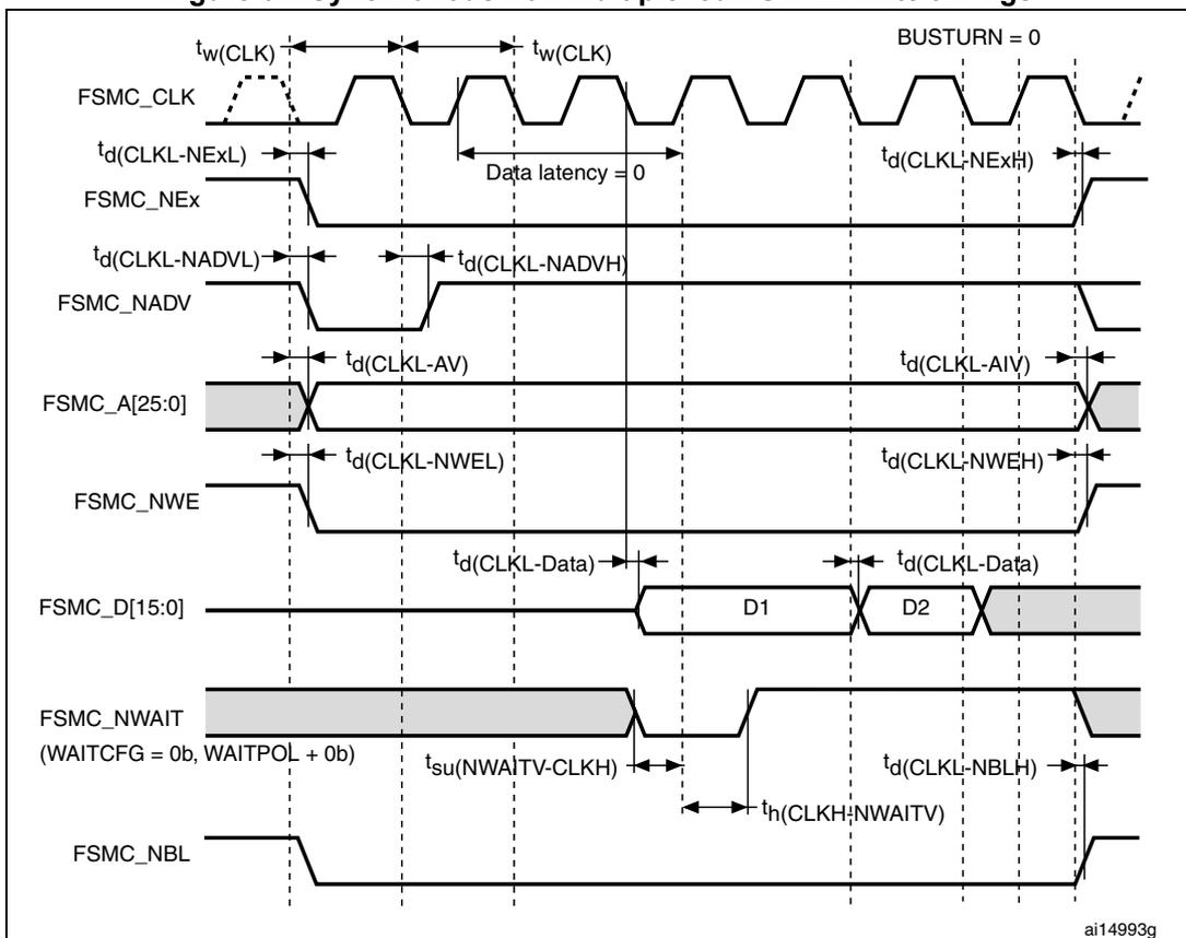
**Table 79. Synchronous non-multiplexed PSRAM write timings<sup>(1)(2)</sup>**
