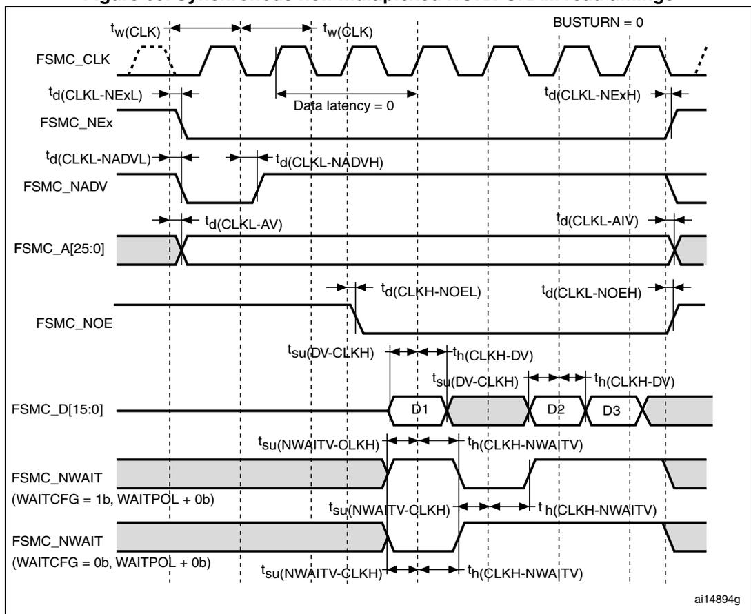
**Table 78. Synchronous non-multiplexed NOR/PSRAM read timings<sup>(1)(2)</sup>**
