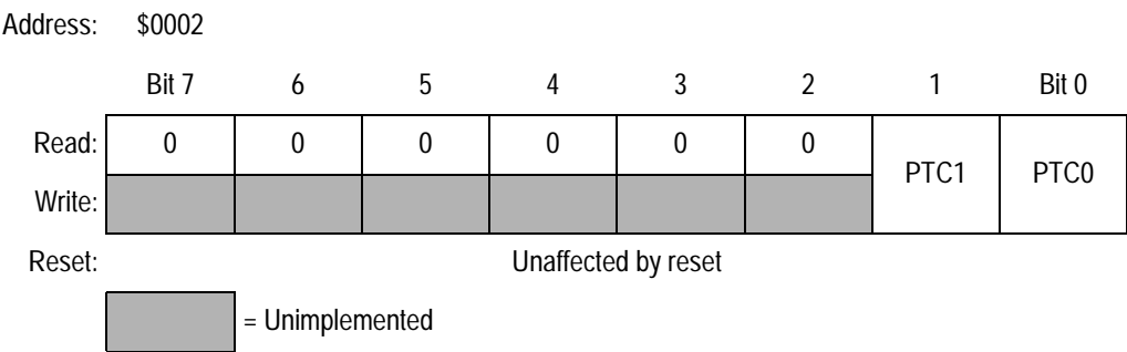
Figure 16-9. Port C Data Register (PTC)
