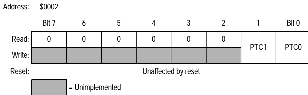
Figure 16-9. Port C Data Register (PTC)
