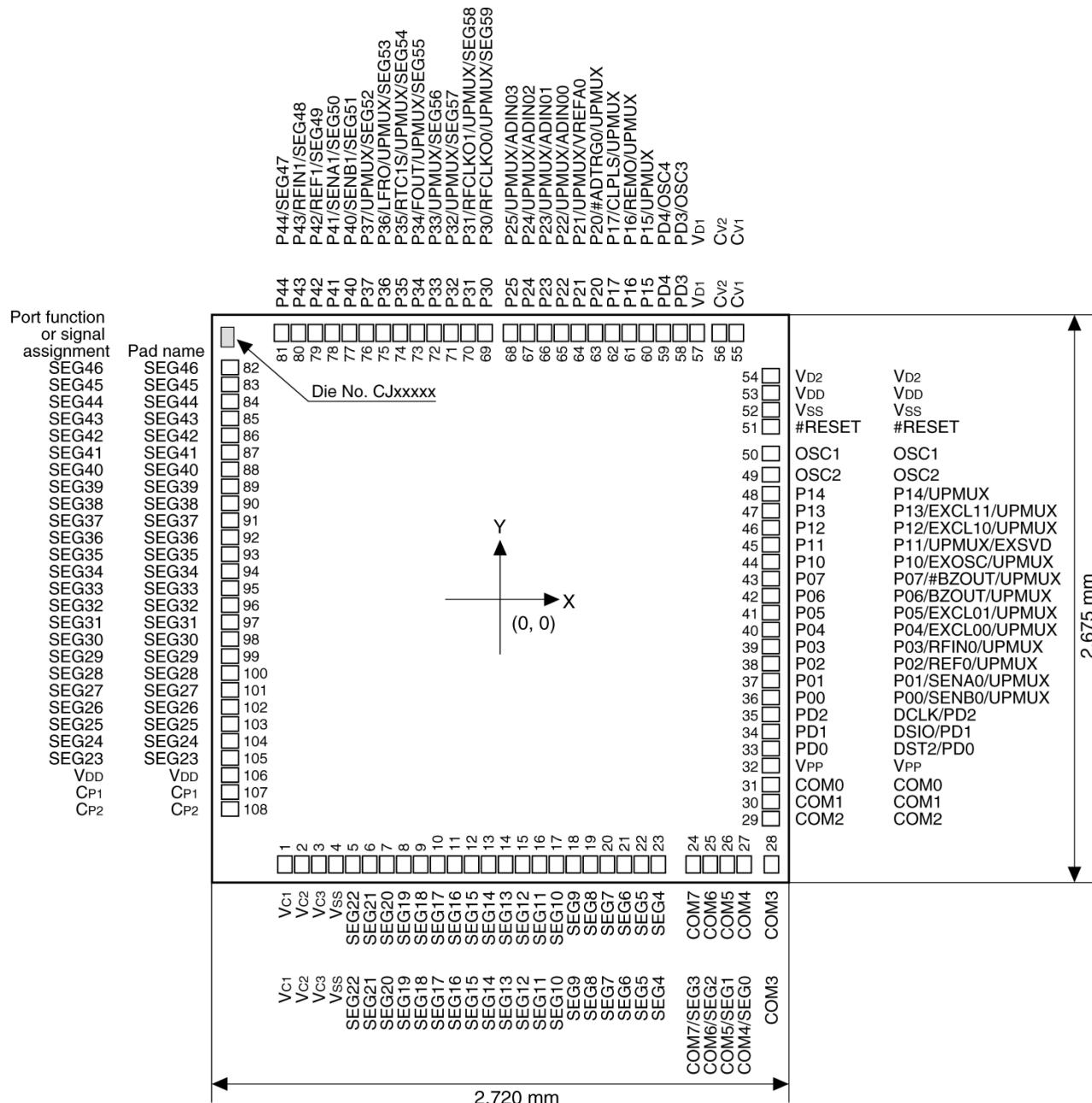
Pad opening No. 1–28, 55–81: X = 68 µm, Y = 80 µm
