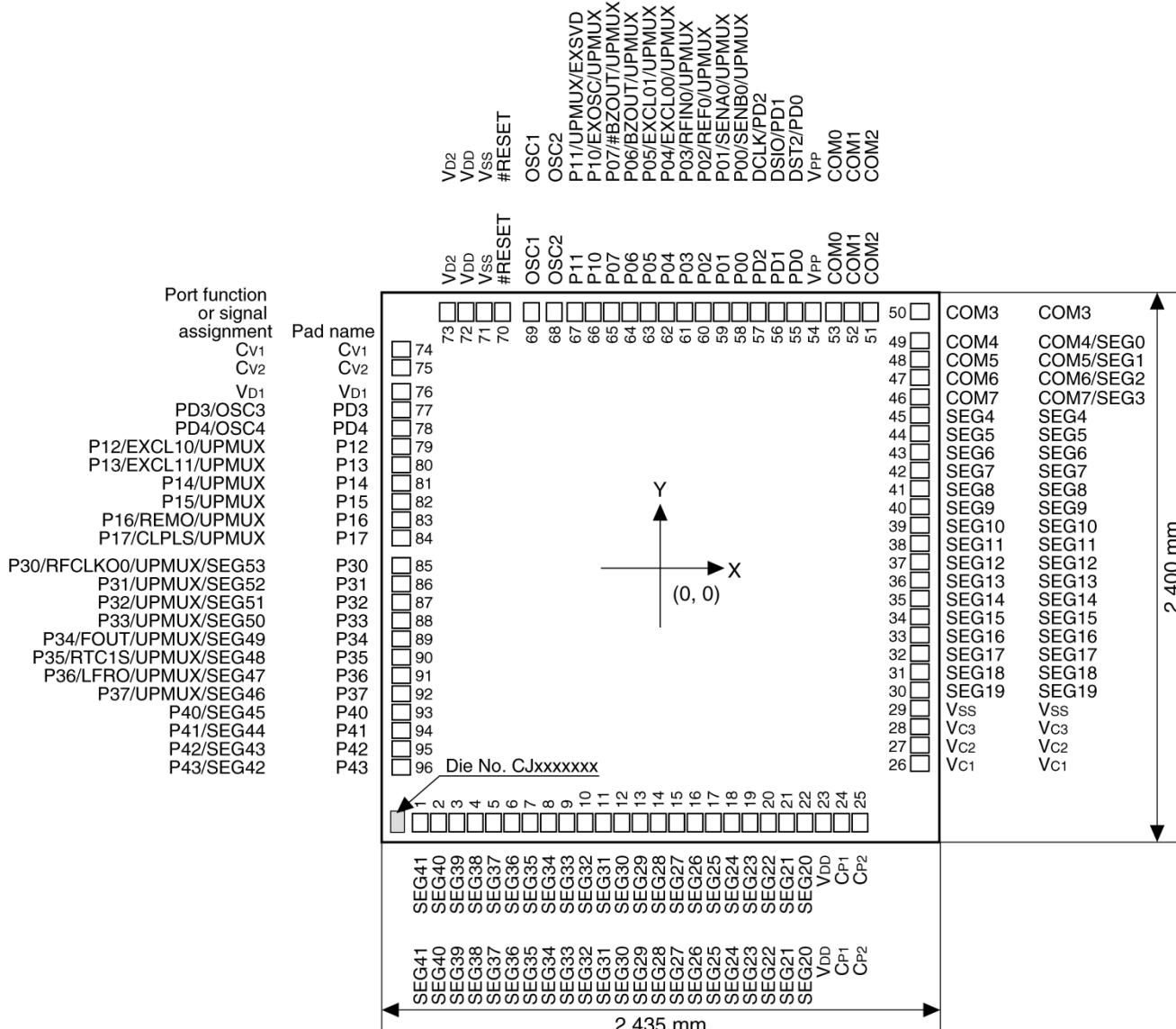
Pad opening No. 1–25, 51–73: X = 68 µm, Y = 80 µm
