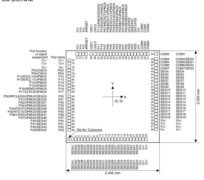
Pad opening No. 1–25, 51–73:  $X = 68 \mu m$ ,  $Y = 80 \mu m$ No. 26–50, 74–96:  $X = 80 \mu m$ ,  $Y = 68 \mu m$
