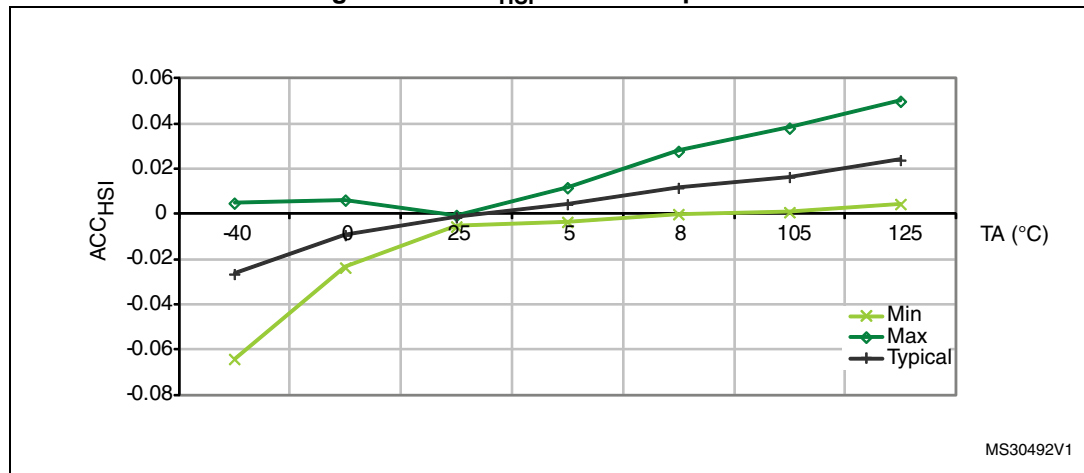
Figure 31. ACC_{HSI} versus temperature
