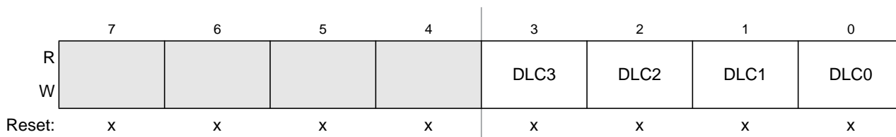
Figure 12-34. Data Length Register (DLR) — Extended Identifier Mapping
