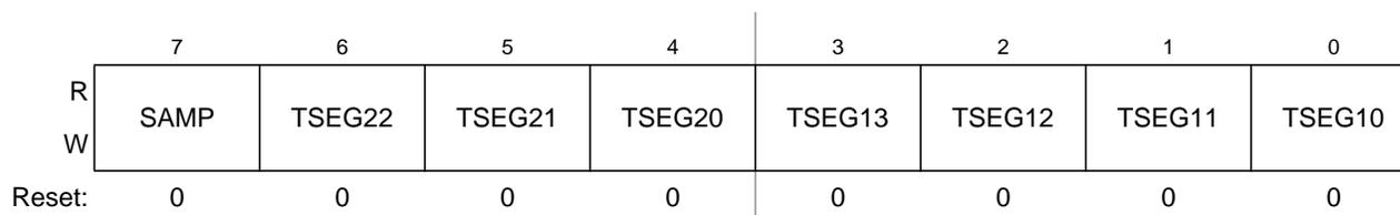
**Figure 12-7. MSCAN Bus Timing Register 1 (CANBTR1)**
