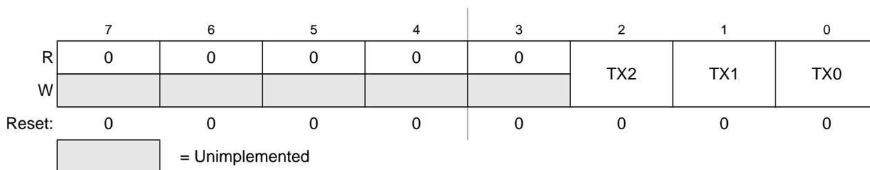
**Figure 12-14. MSCAN Transmit Buffer Selection Register (CANTBSEL)**
