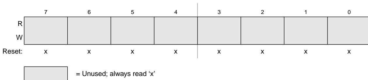
**Figure 12-32. Identifier Register 3 — Standard Mapping**
