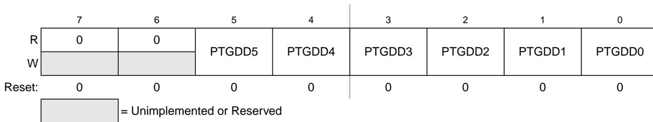
**Figure 6-43. Port G Data Direction Register (PTGDD)**
