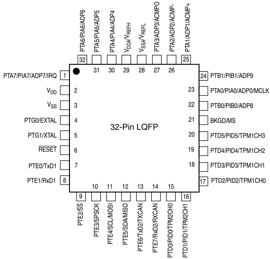
V<sub>REFH</sub> and V<sub>REFL</sub> are internally connected to V<sub>DDA</sub> and V<sub>SSA</sub>, respectively.
