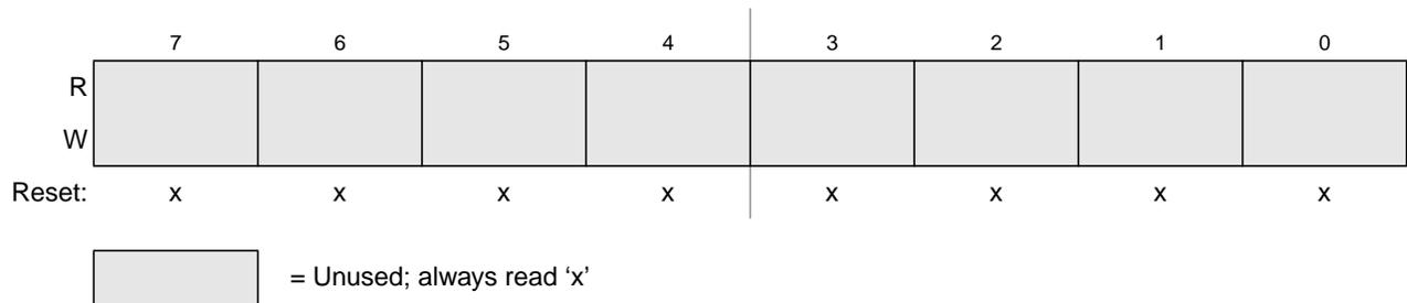
**Figure 12-31. Identifier Register 2 — Standard Mapping**
