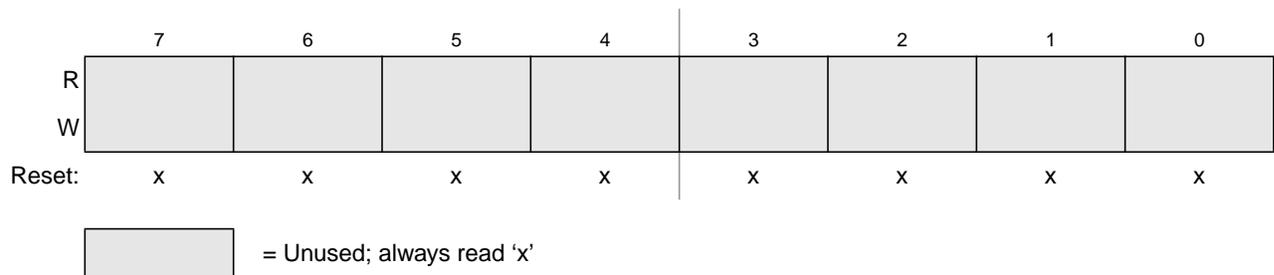
**Figure 12-32. Identifier Register 3 — Standard Mapping**
