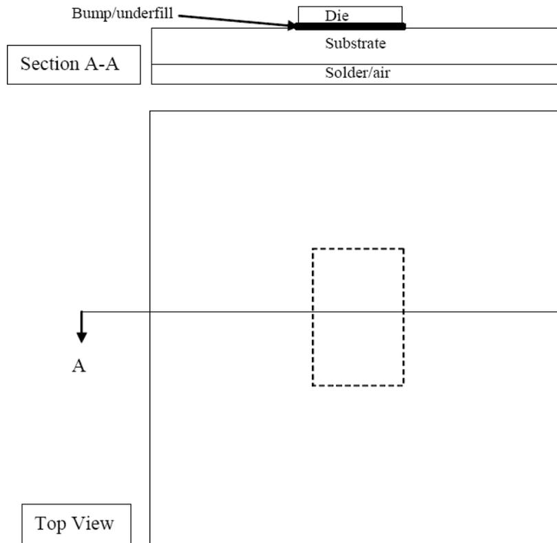
**Figure 72. System-Level Thermal Model for the Chip (Not to Scale)**
