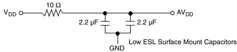
**Figure 75. Chip PLL Power Supply Filter Circuit**
