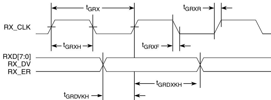
Figure 18. GMII Receive AC Timing Diagram
