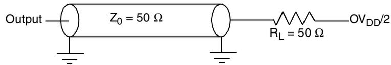
**Figure 45. AC Test Load for the JTAG Interface**
