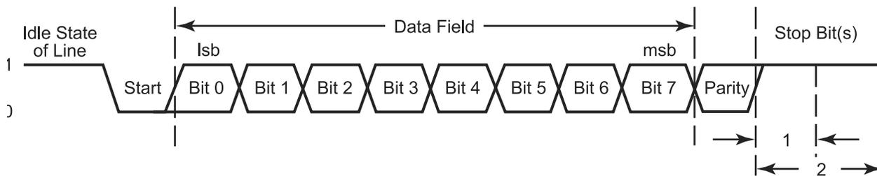
Figure 29. UART-LDD Asynchronous Data Format with Parity
