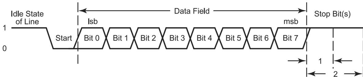
Figure 28. UART-LDD Asynchronous Data Format without Parity
