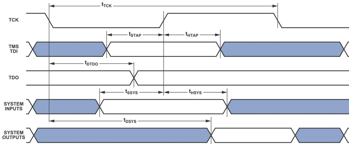
Figure 35. IEEE 1149.1 JTAG Test Access Port
