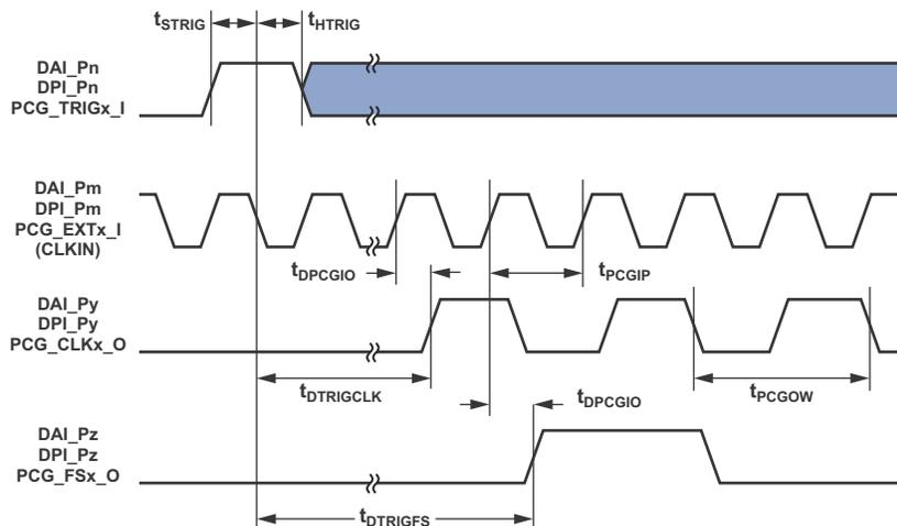
Figure 15. Precision Clock Generator (Direct Pin Routing)
