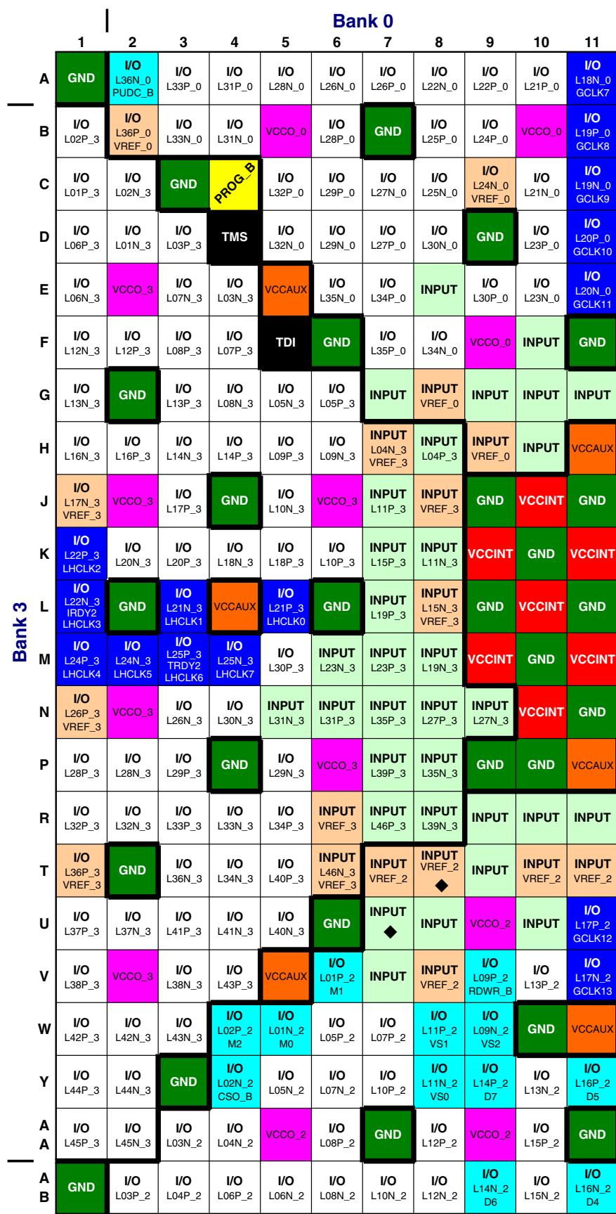
Figure 25: FG484 Package Footprint (Top View)
