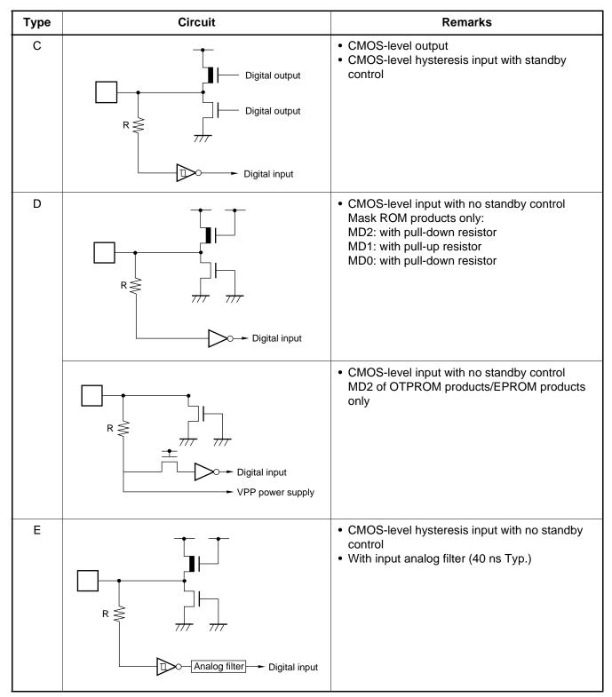
Note: The pull-up and pull-down resistors are always connected, regardless of the state.
