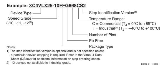
Figure 1: Virtex-4 FPGA Ordering Information
