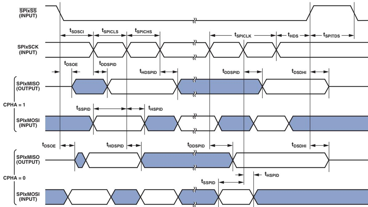
Figure 28. Serial Peripheral Interface (SPI) Port—Slave Timing
