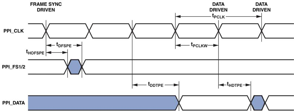
Figure 20. PPI GP Tx Mode with Internal Frame Sync Timing
