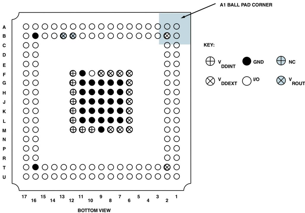
Figure 63. 169-Ball PBGA Ground Configuration (Bottom View)
