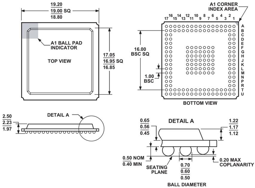
Figure 66. 169-Ball Plastic Ball Grid Array [PBGA]
