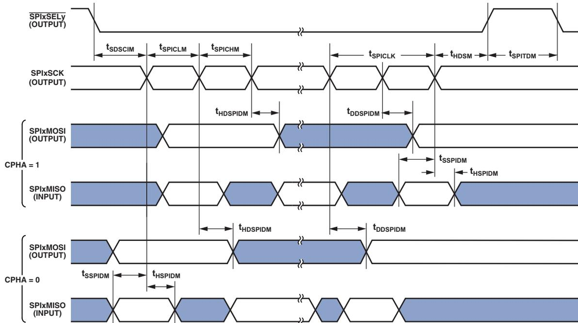
Figure 27. Serial Peripheral Interface (SPI) Port—Master Timing
