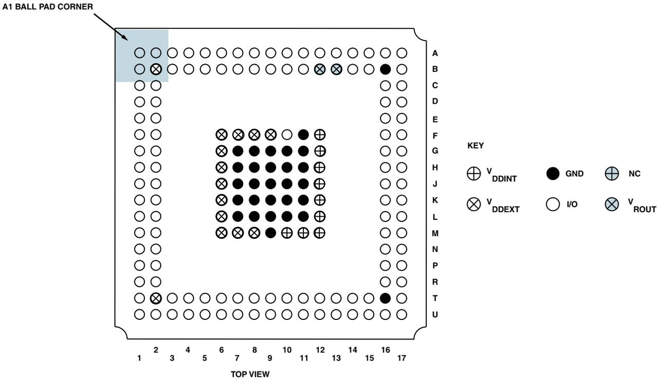
Figure 62. 169-Ball PBGA Ground Configuration (Top View)
