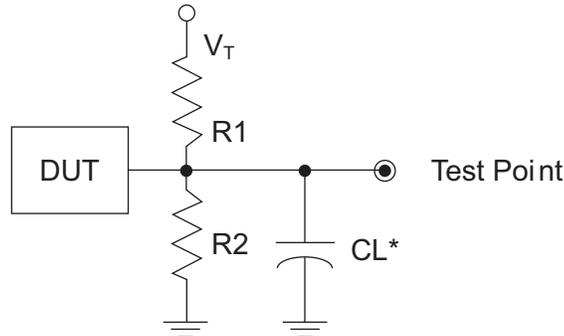
\*CL Includes Test Fixture and Probe Capacitance
