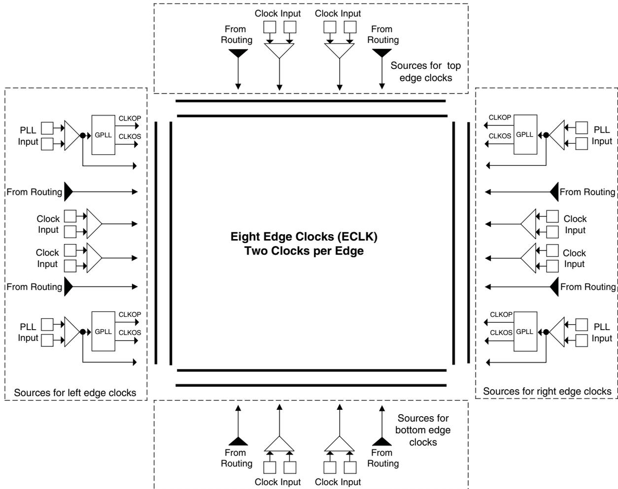
Note: This diagram shows sources for the XP2-17 device. Smaller LatticeXP2 devices have two GPLLs.
