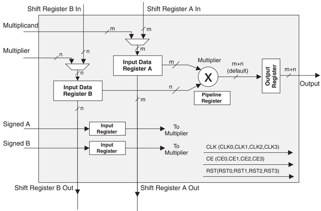
register. Similarly, CE and RST are selected from their four respective sources (CE0, CE1, CE2, CE3 and RST0, RST1, RST2, RST3) at each input register, pipeline register and output register.
