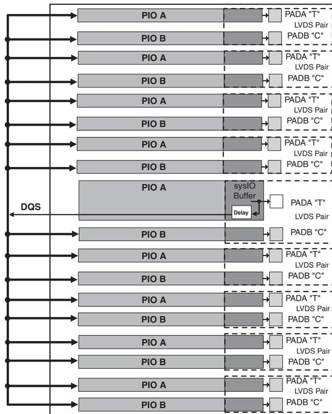
LatticeXP2 devices contain two types of sysIO buffer pairs.
