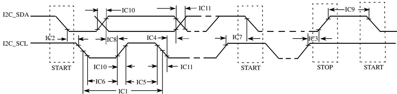
Figure 25. I<sup>2</sup>C Module Timing Diagram
