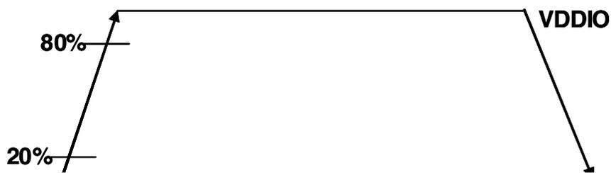
Figure 4. Output Pad Transition Waveform
