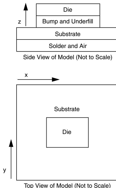
Figure 30. Recommended Thermal Model of MPC7447 and MPC7457
