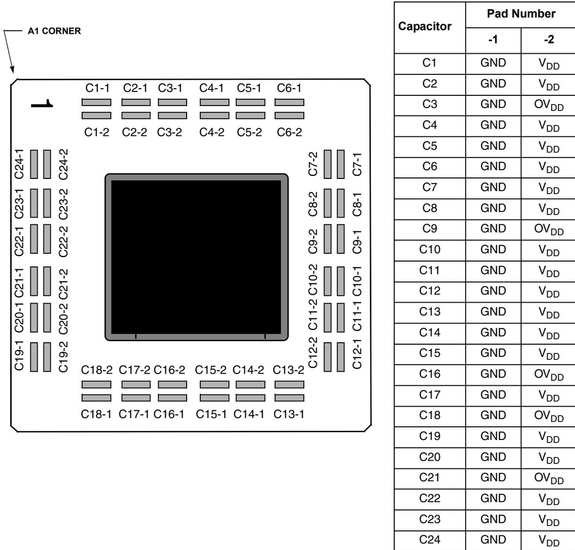
Figure 21. Substrate Bypass Capacitors for the MPC7447, 360 CBGA
