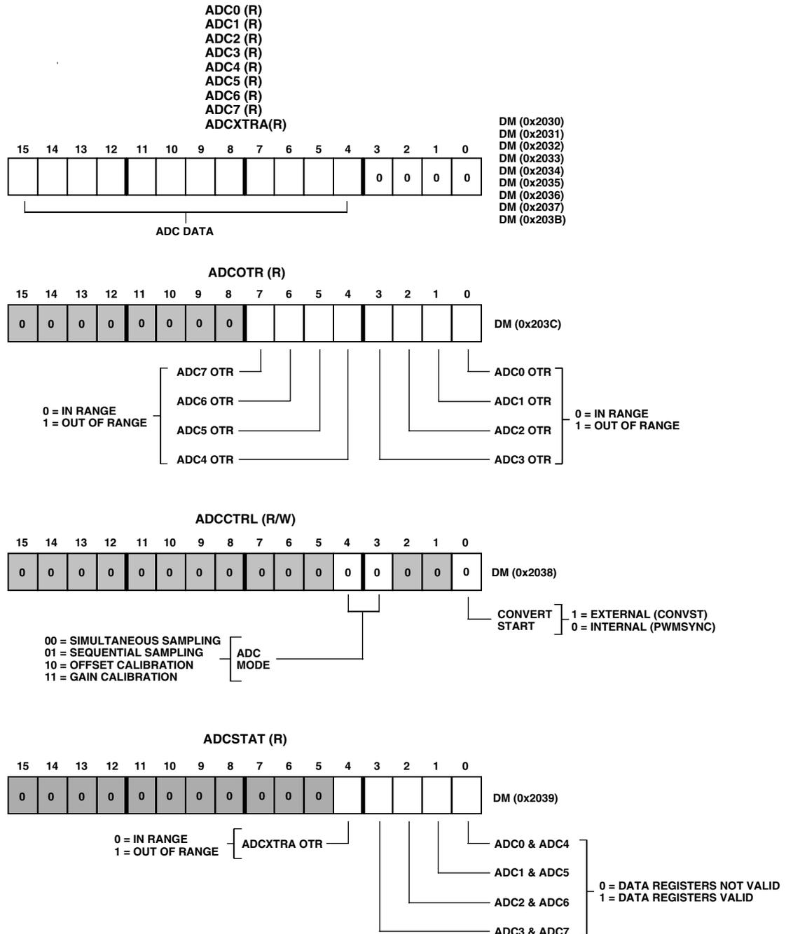
Figure 35. Structure of Registers of the ADCM401
