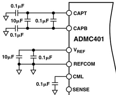
Figure 20. Recommended Capacitor Decoupling Networks for the ADCM401
