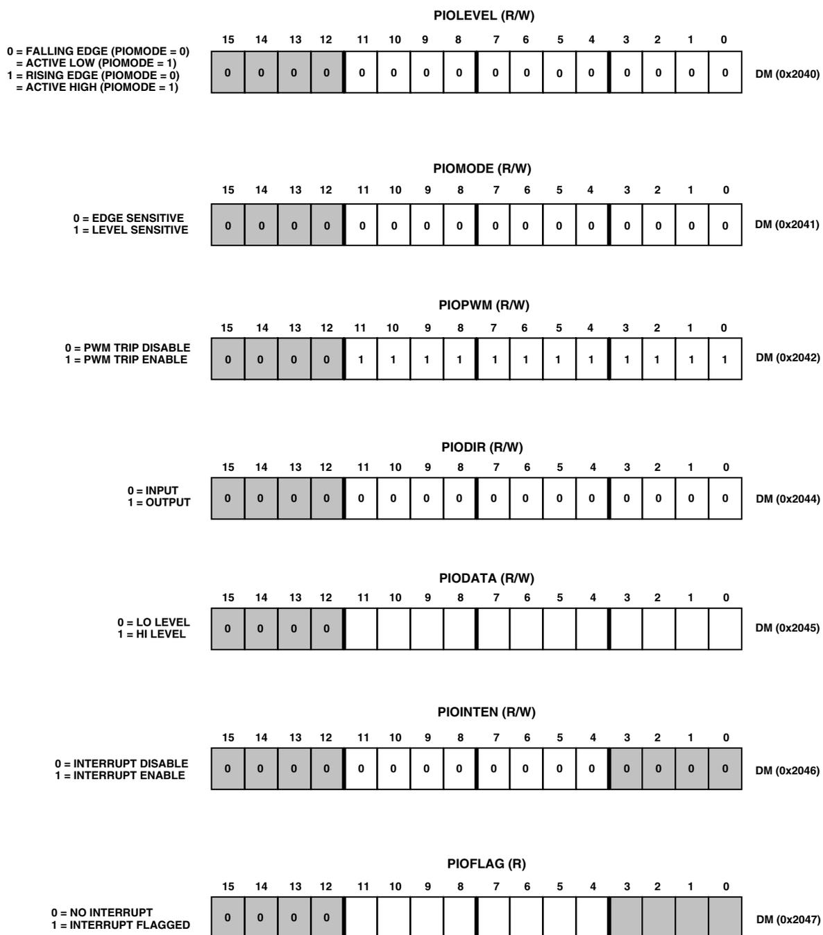
Figure 39. Structure of Registers of ADC401
