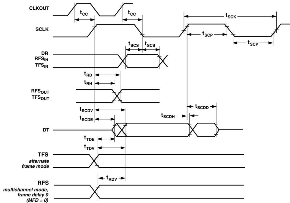
Figure 6. Serial Ports
