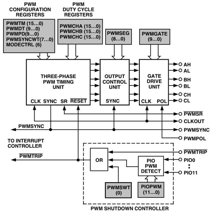
Figure 21. Overview of the ADCM401 PWM Controller
