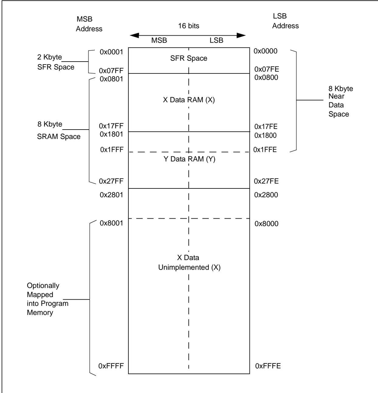
**FIGURE 3-7: DATA SPACE FOR MCU AND DSP (MAC CLASS) INSTRUCTIONS EXAMPLE**
