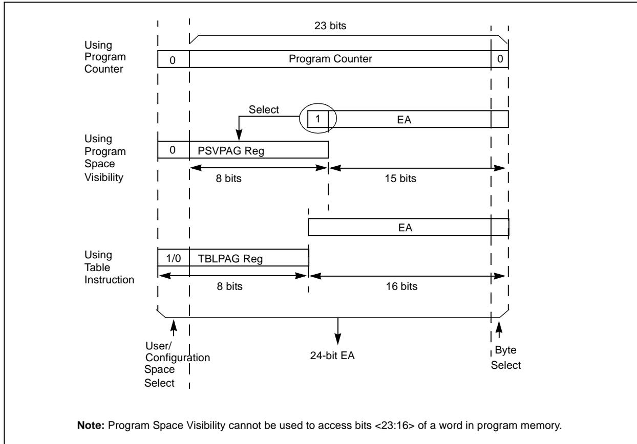
**FIGURE 3-5: DATA SPACE WINDOW INTO PROGRAM SPACE OPERATION**
