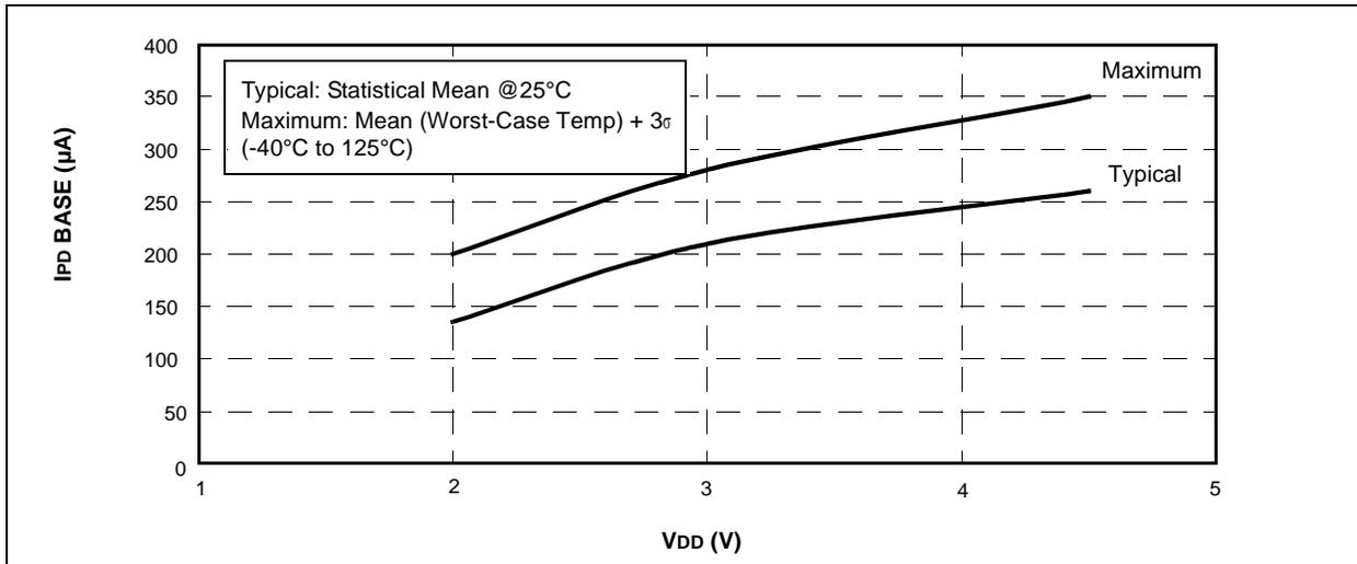
**FIGURE 16-28: PIC16HV610/616 I<sub>PD</sub> COMPARATOR (SINGLE ON) vs. V<sub>DD</sub>**
