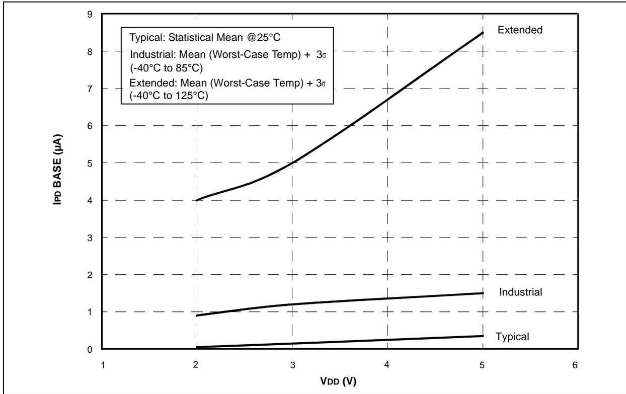
FIGURE 16-11: PIC16F610/616 IPD COMPARATOR (SINGLE ON) vs. VDD
