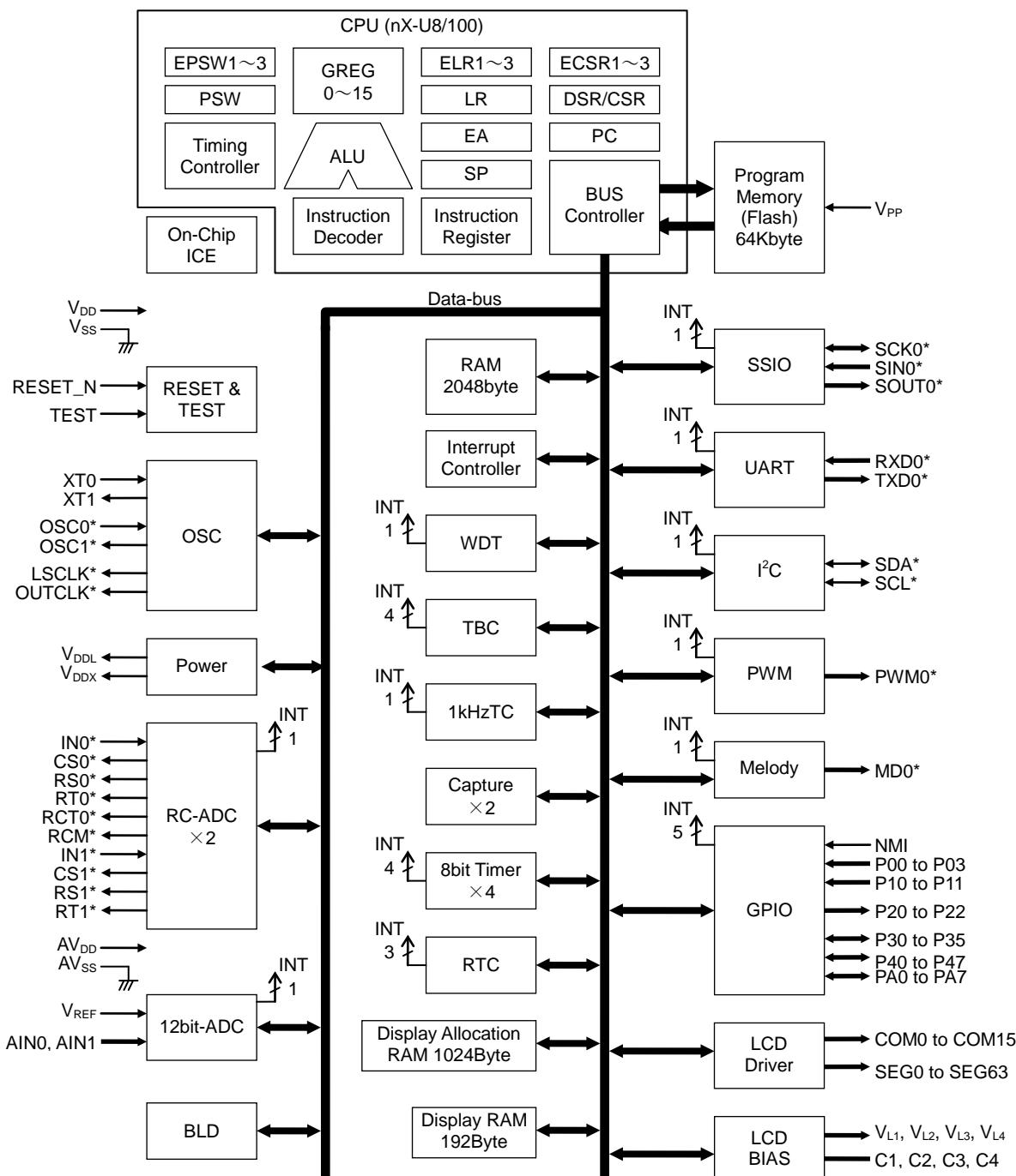
**Figure 1 ML610Q431 Block Diagram**
