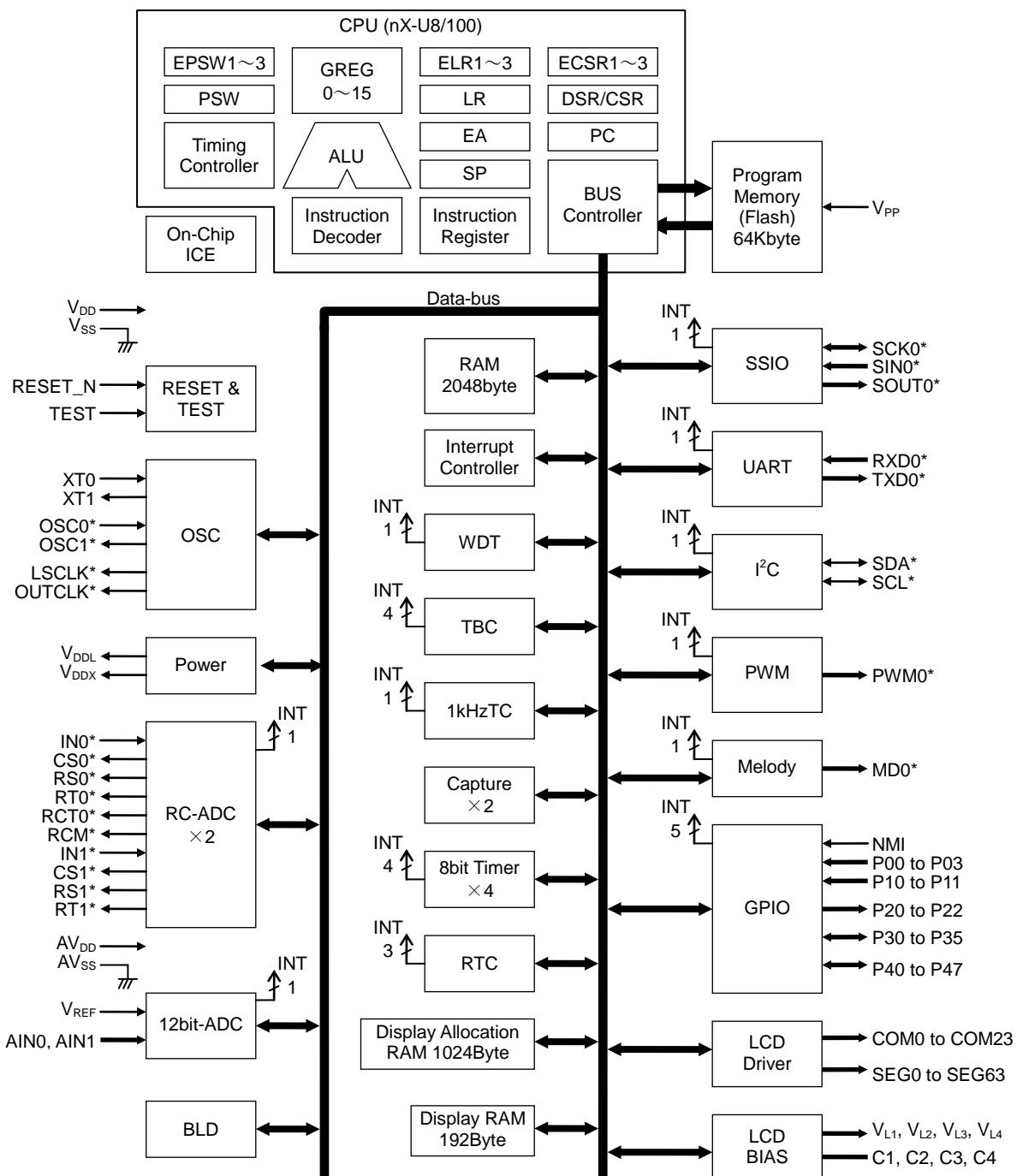
Figure 2 ML610Q432 Block Diagram
