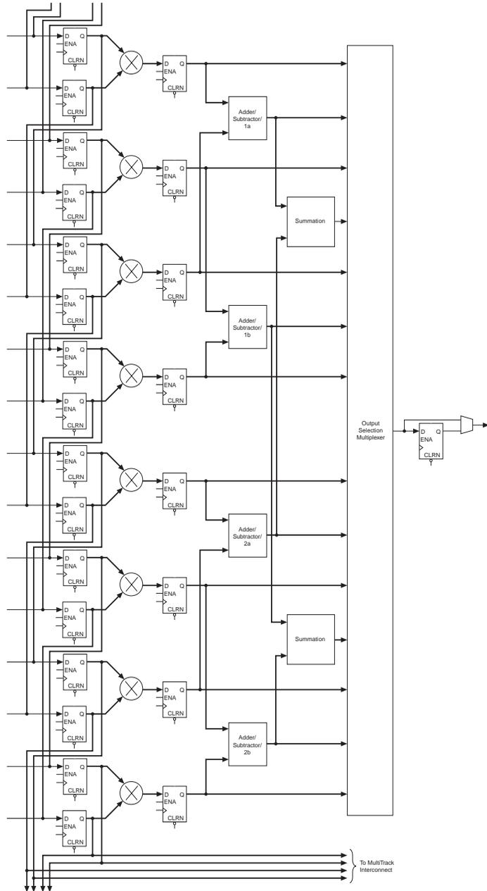
Figure 4–32. Multiplier Sub-Blocks Using Input Shift Register Connections *Note (1)*
