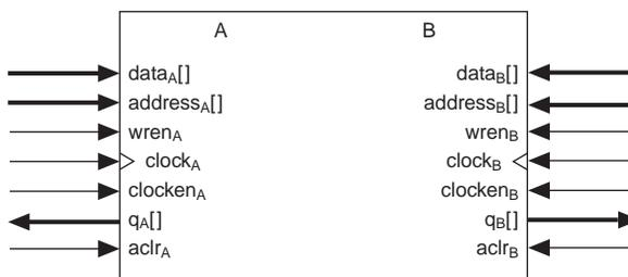
In addition to true dual-port memory, the memory blocks support simple dual-port and single-port RAM. Simple dual-port memory supports a simultaneous read and write and can either read old data before the write
