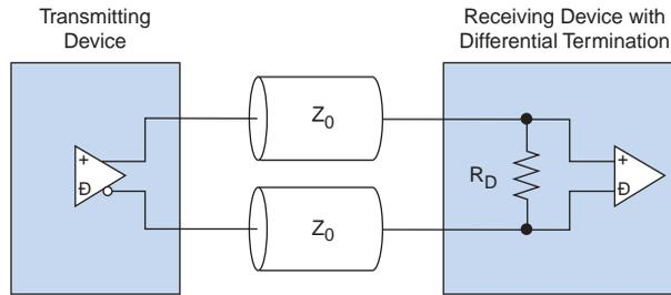
I/O banks on the left and right side of the device support LVDS receiver (far-end) differential termination.
