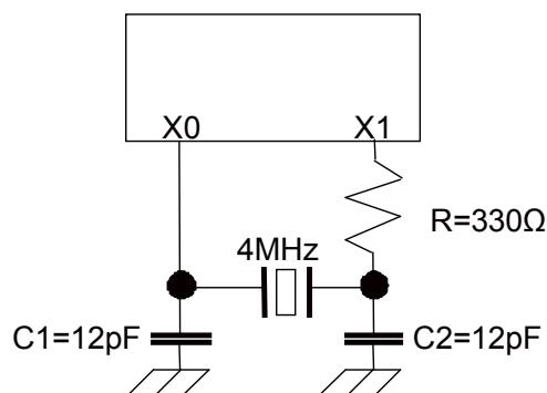
Note: If it is impossible to start the oscillation within or equal to 20ms when starting from the oscillation stop state, the clock supervisor performs a detection of oscillation stop and moves to the fail safe operation.
