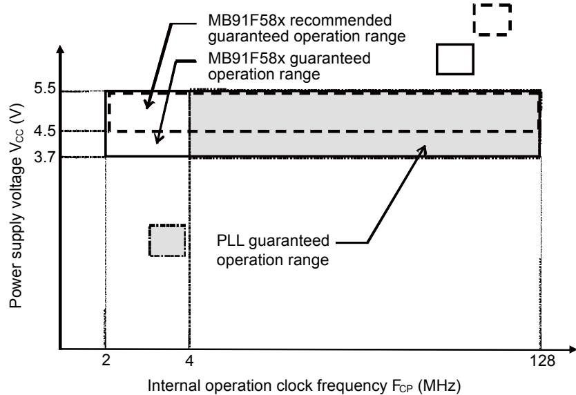
Note: The CPU will be reset at the power supply voltage of the low-voltage detection setting voltage or less.
