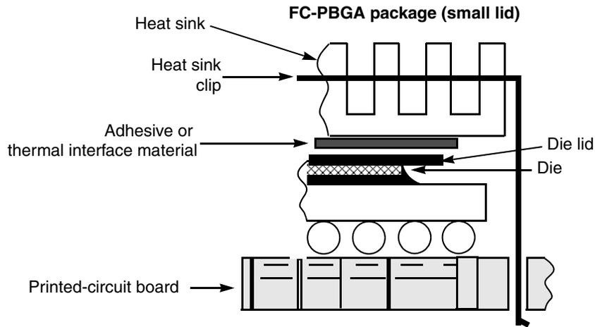
**Figure 62. Exploded cross-sectional view—FC-PBGA (with lid) package**
