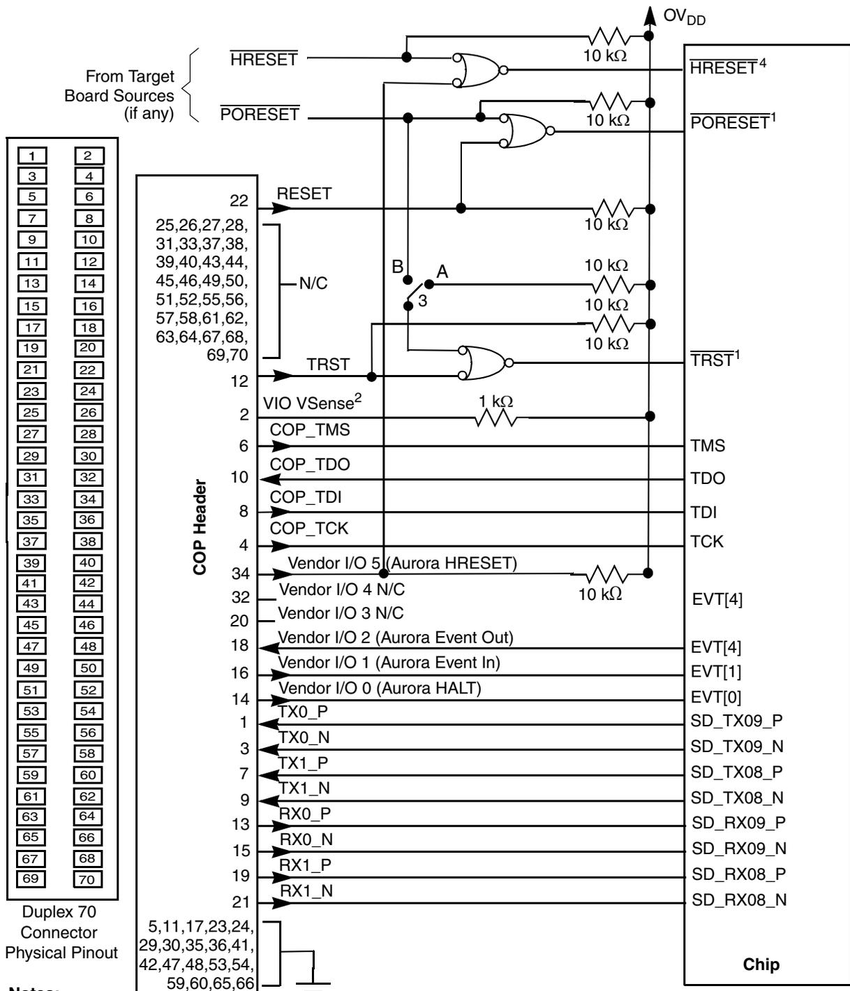
Figure 60. Aurora 70 pin connector duplex interface connection
