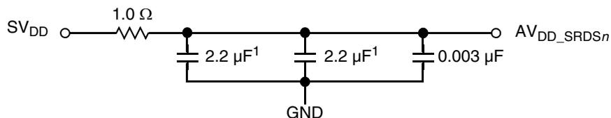
Figure 52. SerDes PLL power supply filter circuit
