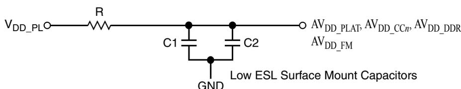
Figure 51. PLL power supply filter circuit
