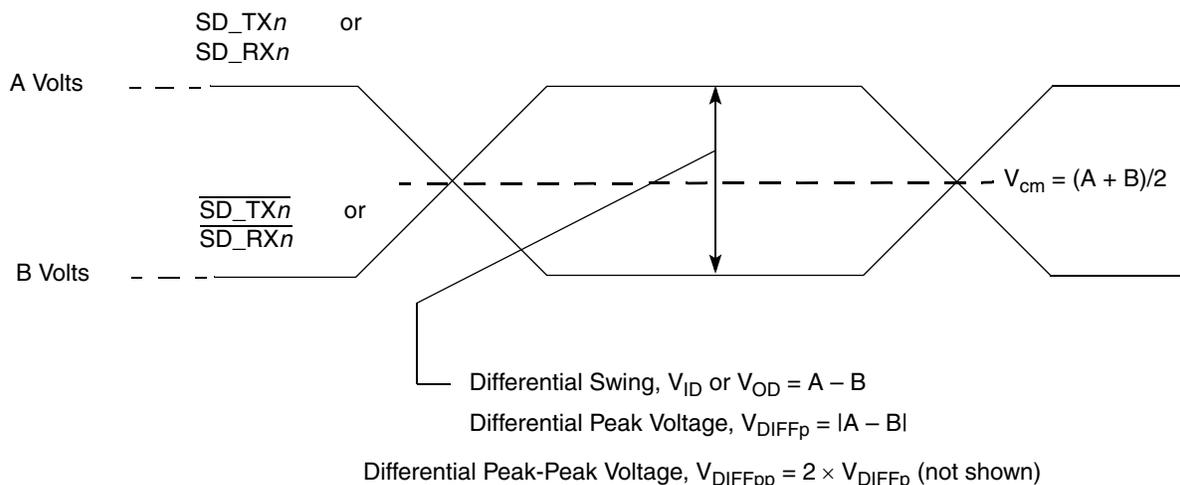
**Figure 35. Differential voltage definitions for transmitter or receiver**
