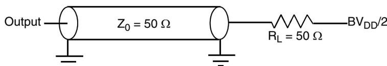
**Figure 23. Enhanced local bus AC test load**
