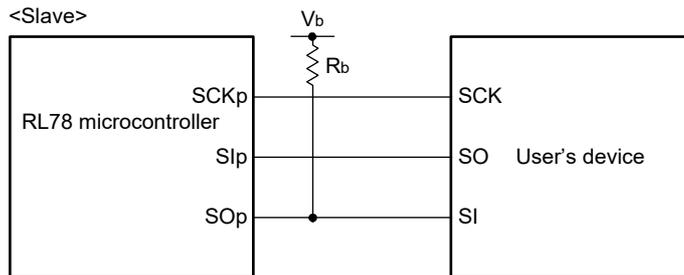
**Remark 1.** R<sub>b</sub>[Ω]: Communication line (SO<sub>p</sub>) pull-up resistance, C<sub>b</sub>[F]: Communication line (SO<sub>p</sub>) load capacitance, V<sub>b</sub>[V]: Communication line voltage
