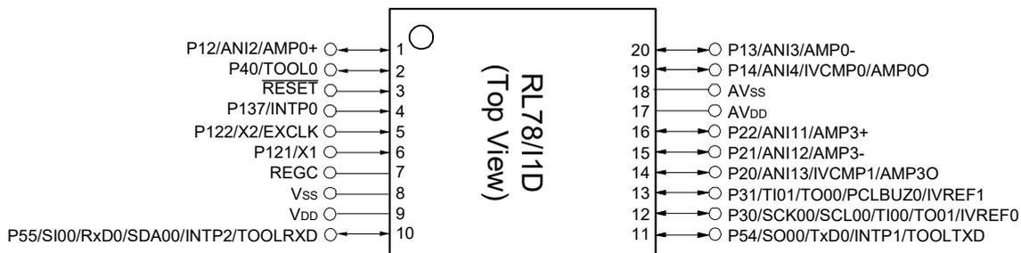
**Caution 1.** Connect the REGC pin to Vss pin via a capacitor (0.47 to 1 μF).
