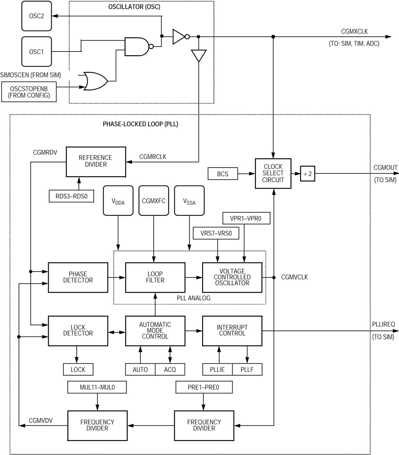
**Figure 4-1. CGM Block Diagram**
