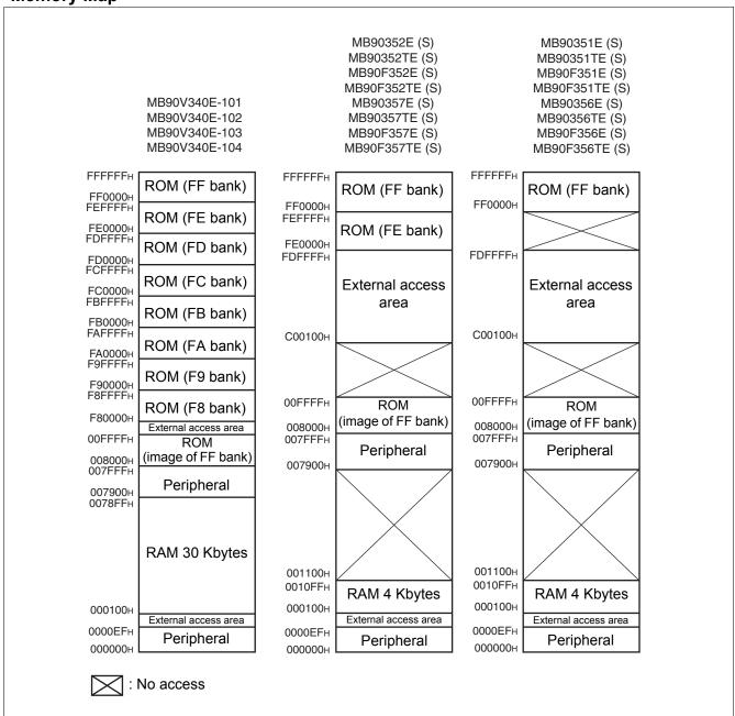
Note: The high-order portion of bank 00 gives the image of the FF bank ROM to make the small model of the C compiler effective. Since the low-order 16 bits are the same, the table in ROM can be referenced without using the far specification in the pointer declaration.
