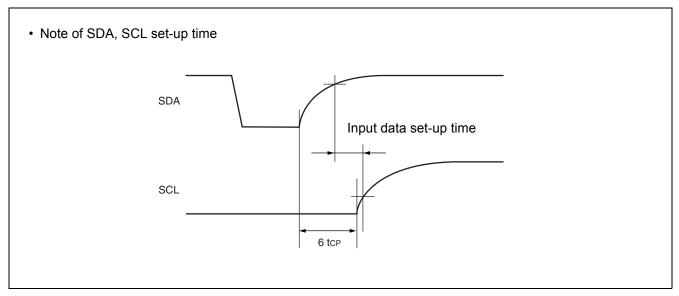
Note: The rating of the input data set-up time in the device connected to the bus cannot be satisfied depending on the load capacitance or pull-up resistor.
