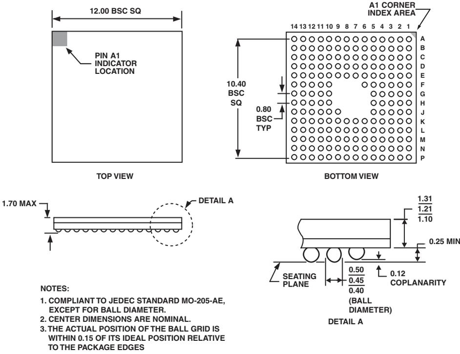
Figure 67. 182-Ball Chip Scale Package Ball Grid Array [CSP\_BGA]
