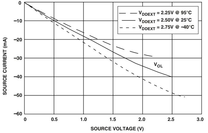
Figure 46. Drive Current F (Low  $V_{DDEXT}$ )
