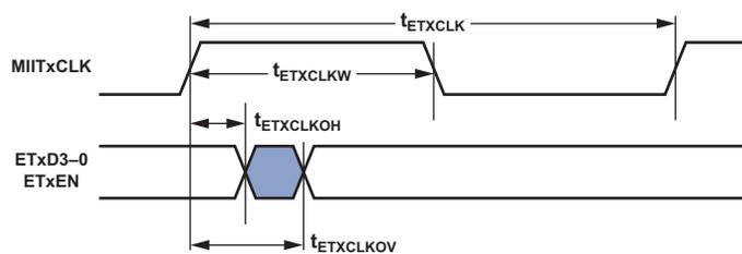
Figure 31. 10/100 Ethernet MAC Controller Timing: MII Transmit Signal
