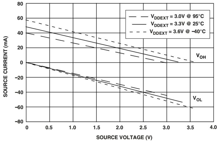
Figure 45. Drive Current E (High  $V_{DDEXT}$ )
