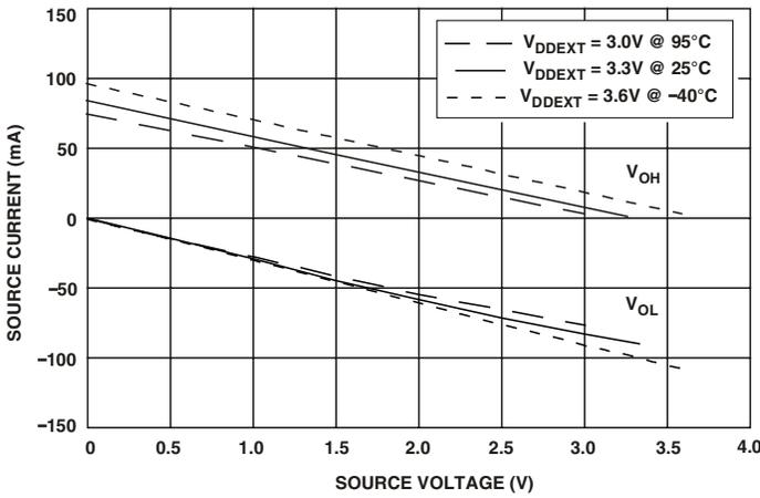
Figure 43. Drive Current D (High  $V_{DDEXT}$ )
