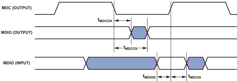
Figure 35. 10/100 Ethernet MAC Controller Timing: MII Station Management
