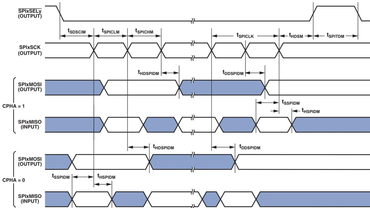
Figure 24. Serial Peripheral Interface (SPI) Port—Master Timing
