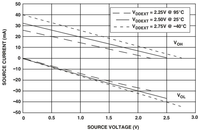
Figure 44. Drive Current E (Low  $V_{DDEXT}$ )
