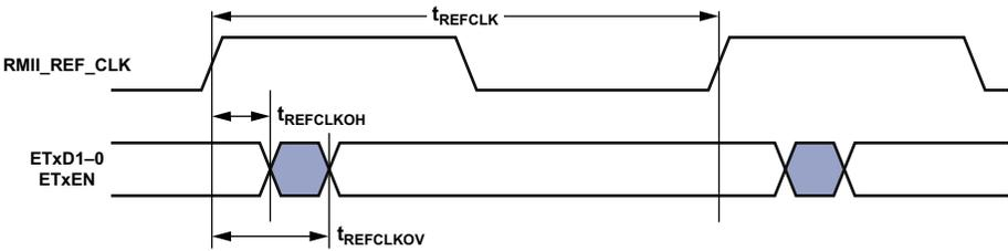
Figure 33. 10/100 Ethernet MAC Controller Timing: RMII Transmit Signal
