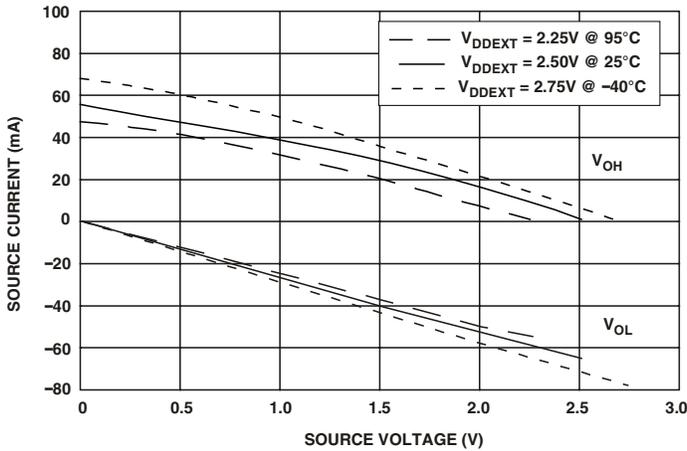
Figure 42. Drive Current D (Low  $V_{DDEXT}$ )
