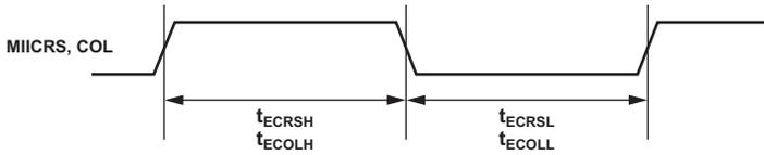
Figure 34. 10/100 Ethernet MAC Controller Timing: Asynchronous Signal
