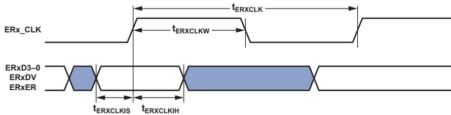
Figure 30. 10/100 Ethernet MAC Controller Timing: MII Receive Signal
