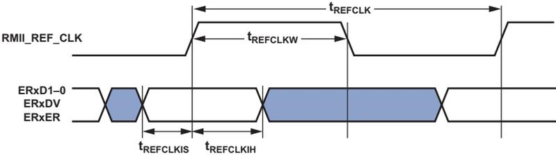
Figure 32. 10/100 Ethernet MAC Controller Timing: RMII Receive Signal
