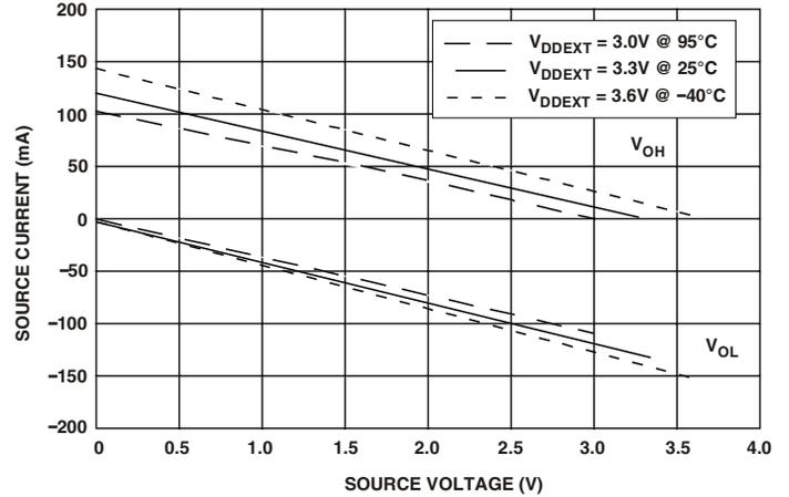
Figure 39. Drive Current B (High  $V_{DDEXT}$ )
