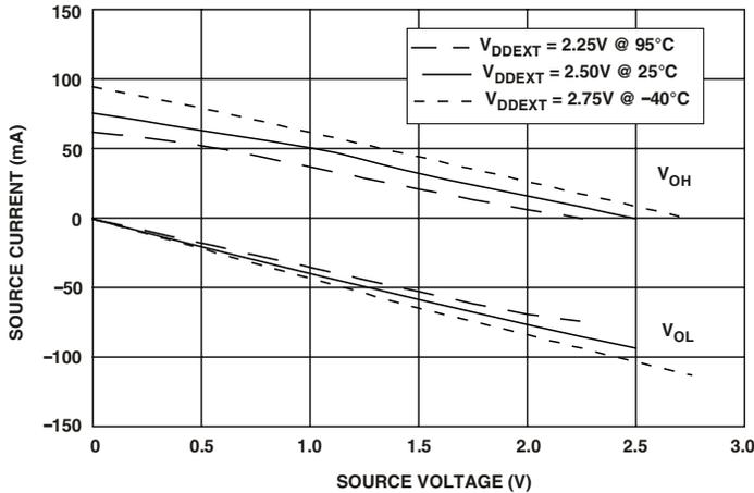
Figure 38. Drive Current B (Low  $V_{DDEXT}$ )
