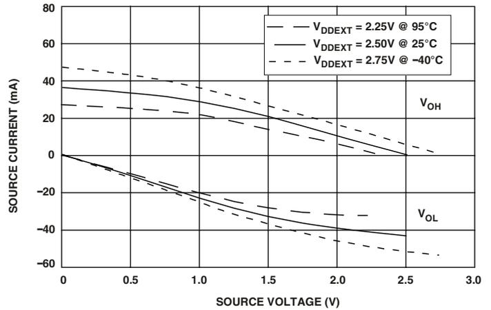
Figure 40. Drive Current C (Low  $V_{DDEXT}$ )
