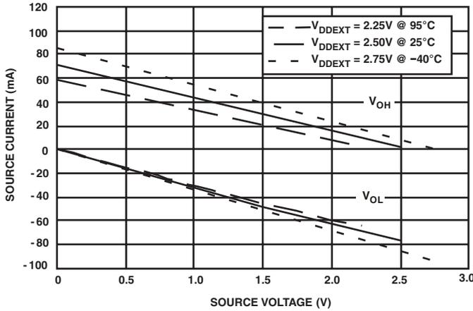
Figure 36. Drive Current A (Low  $V_{DDEXT}$ )
