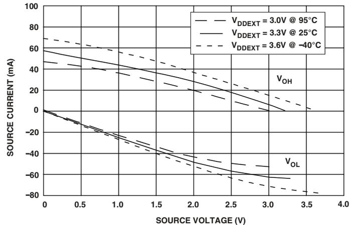
Figure 41. Drive Current C (High  $V_{DDEXT}$ )
