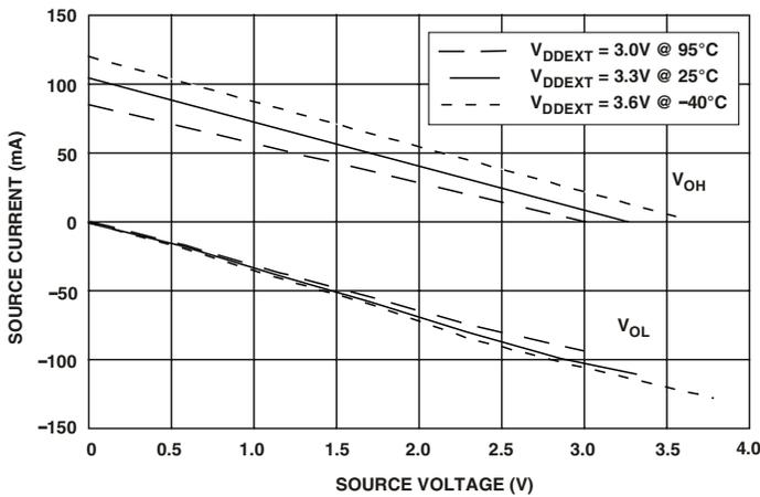
Figure 37. Drive Current A (High  $V_{DDEXT}$ )
