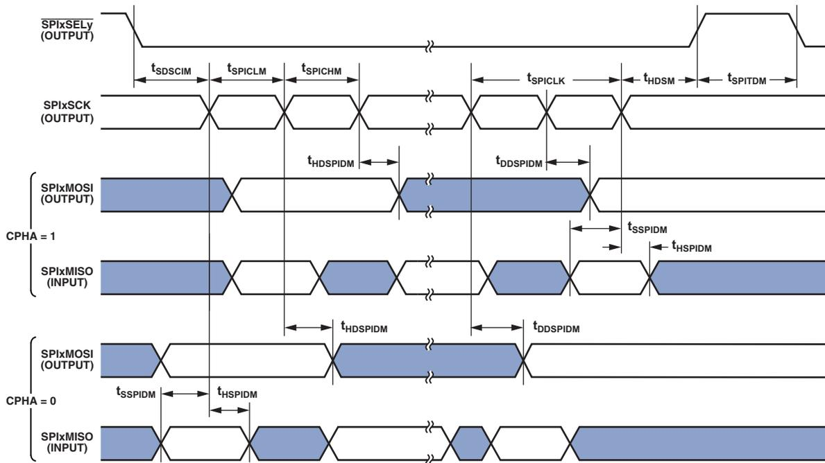
Figure 24. Serial Peripheral Interface (SPI) Port—Master Timing
