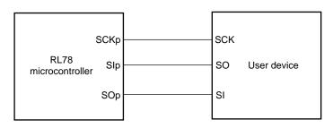
CSI mode connection diagram (during communication at same potential)
