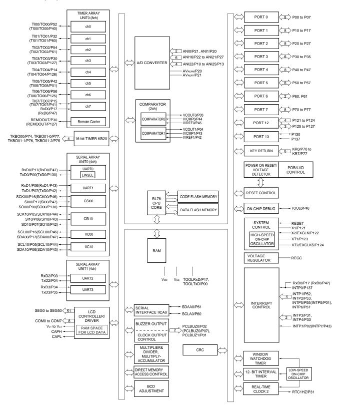
Remark Functions in parentheses in the above figure can be assigned via settings in the peripheral I/O redirection register (PIOR). See Figure 4-8 Format of Peripheral I/O Redirection Register (PIOR) in the RL78/L13 User's Manual.
