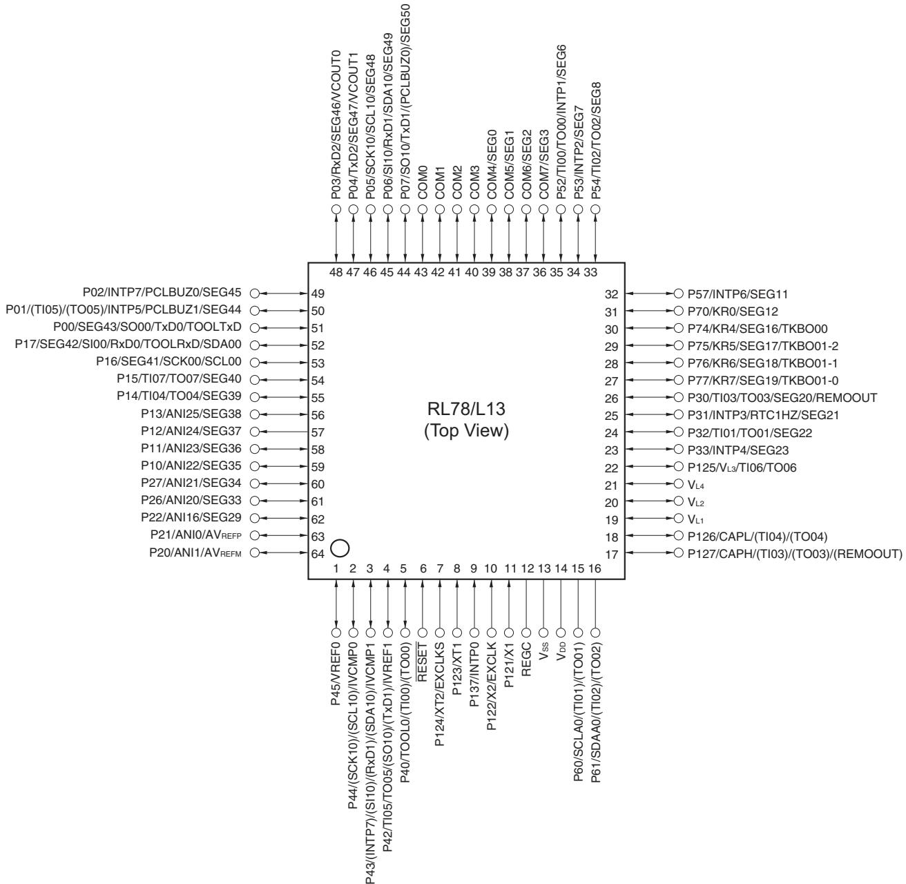
**Caution Connect the REGC pin to V<sub>ss</sub> via a capacitor (0.47 to 1  $\mu$ F).**
