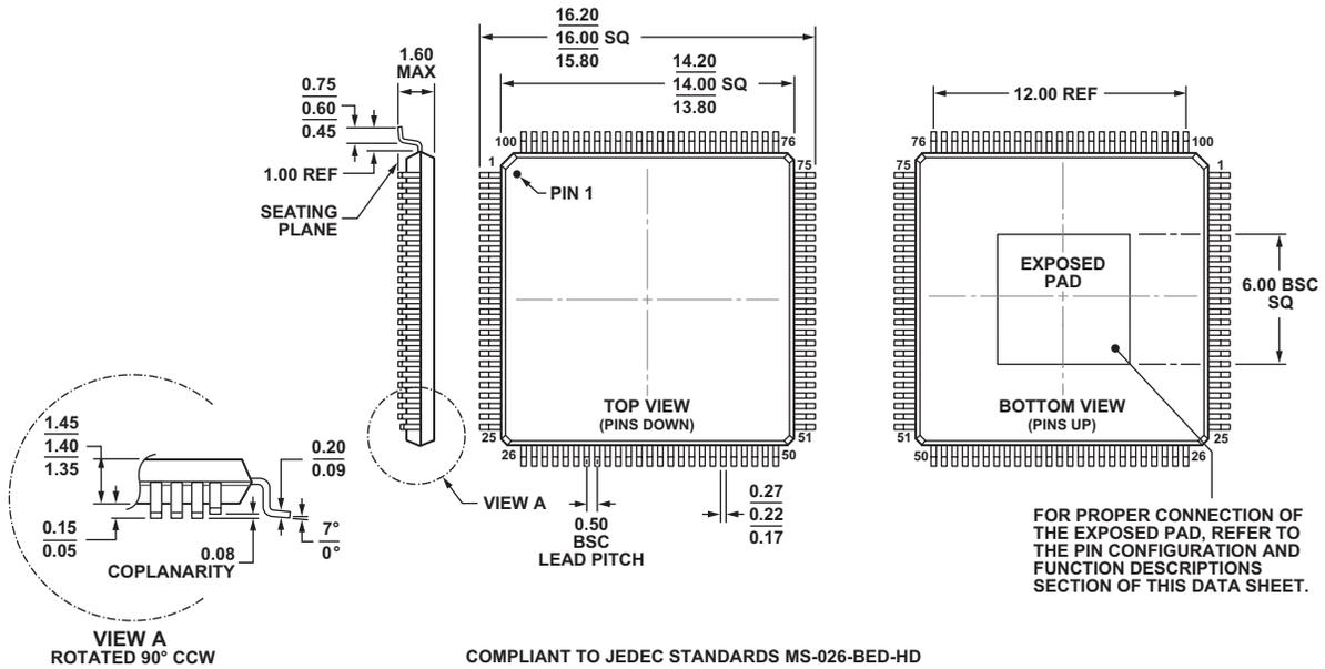
Figure 58. 100-Lead Low Profile Quad Flat Package, Exposed Pad [LQFP\_EP<sup>1</sup>] (SW-100-2)
