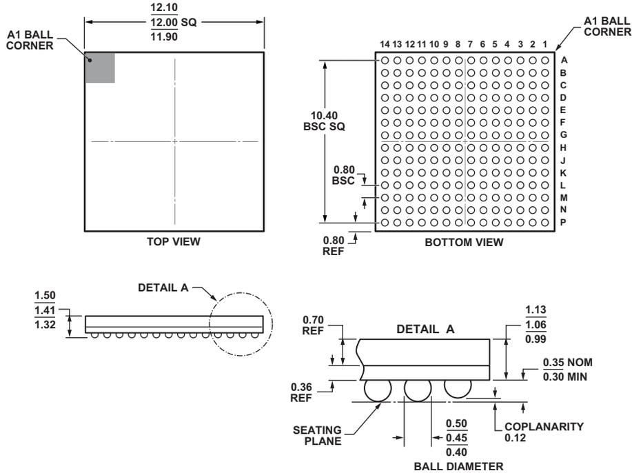
Figure 59. 196-Ball Chip Scale Package, Ball Grid Array [CSP\_BGA] (BC-196-8)
