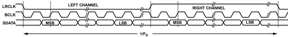
Figure 32. PS Mode—16 Bits to 24 Bits Per Channel
