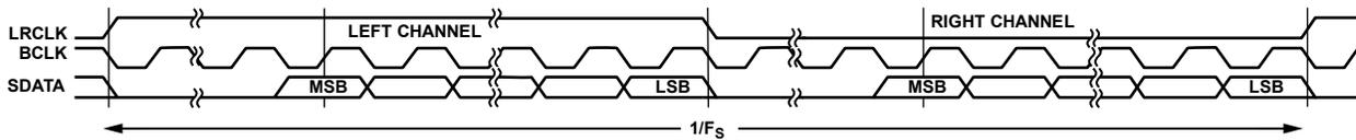
Figure 34. Right-Justified Mode—16 Bits to 24 Bits Per Channel
