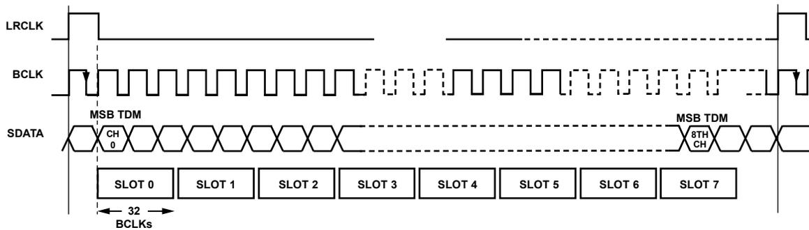
Figure 36. TDM Mode with Pulse Word Clock
